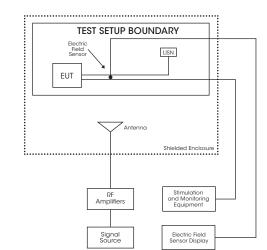
Figure R\$103.1 Test Equipment Configurations
