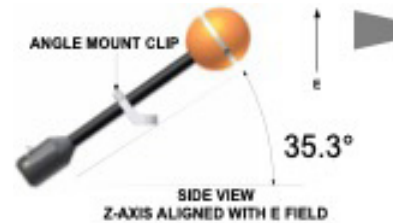
Figure 1: Side View: Z-Axis Aligned with E Field
