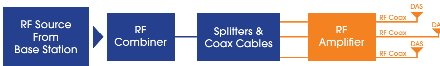
Figure 2: Block diagram of a Passive DAS System
