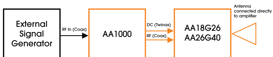
Figure 4: AA-Series Equipment Block Diagram with Provided Equipment Highlighted
