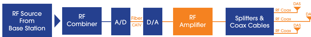
Figure 3: Block diagram of a Hybrid DAS System
