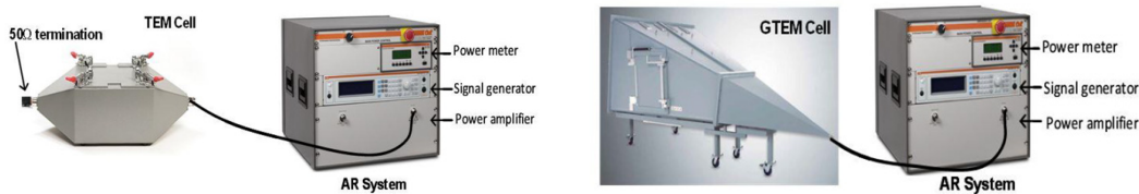
Figure 1: TEM cell immunity test set-up
