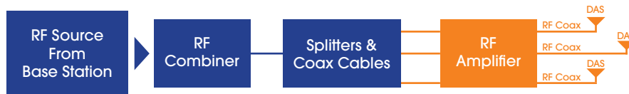
Figure 2: Block diagram of a Passive DAS System
